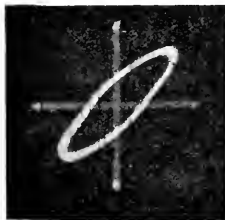
FIGS. 6, 7, 8 AND 9.—PHASE DIFFERENCES IN ALTERNATING CIRCUITS.
